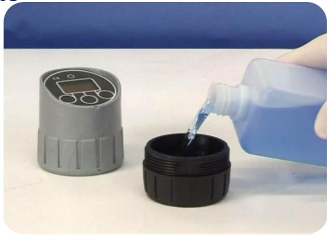
Add Reagent A to the top line (note; for lowest range test, volume is increased – use syringe)
